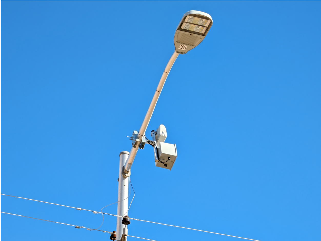
Figure 8: Detail of a ShotSpotter sensor
