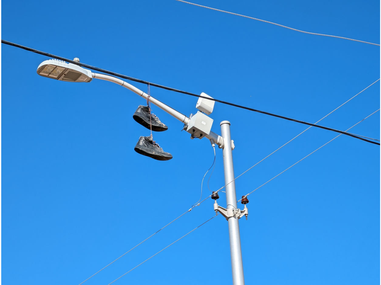
Figure 1: ShotSpotter sensor on light pole
