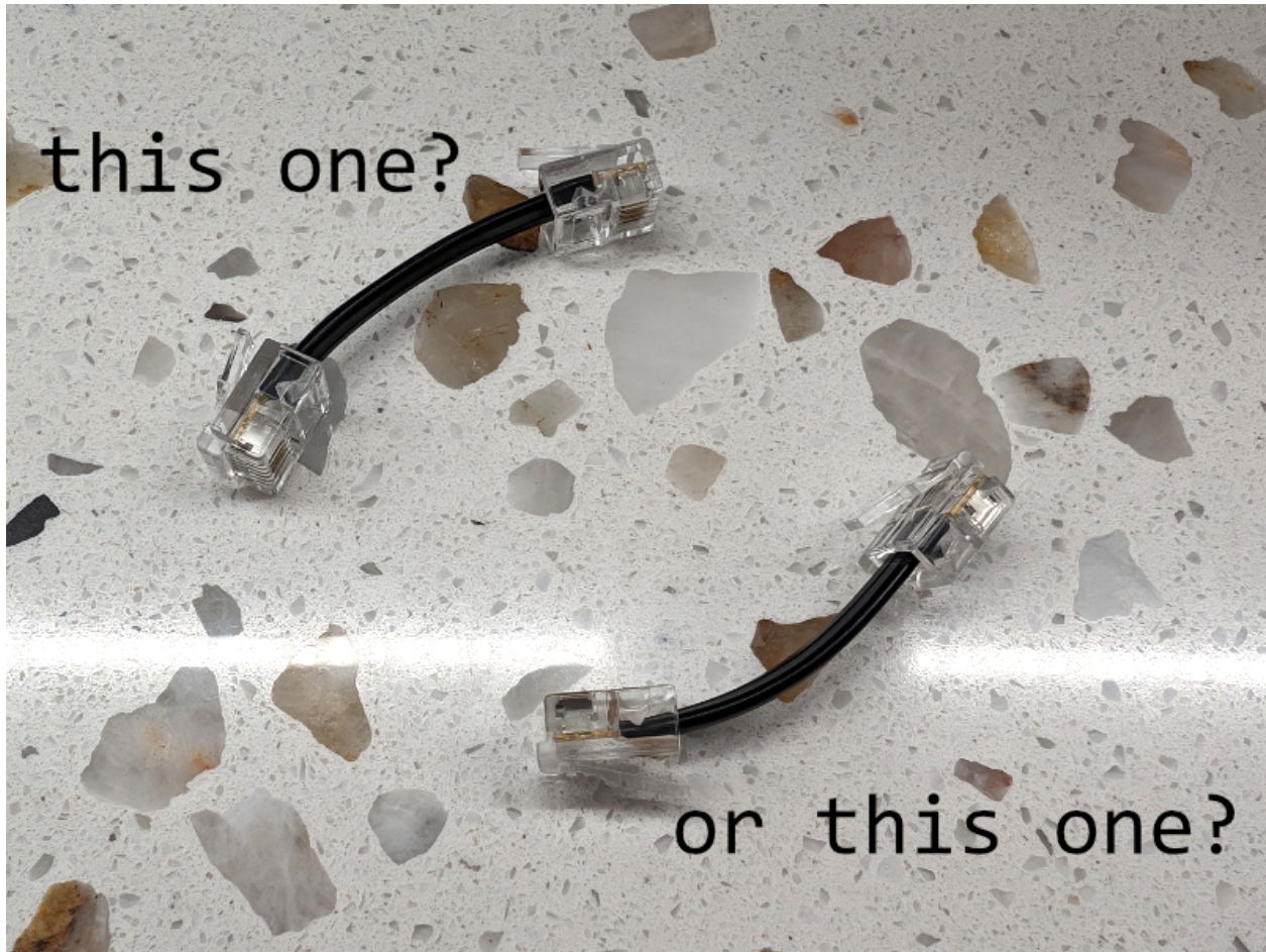
Figure 1: two phone cables, terminated opposite ways
